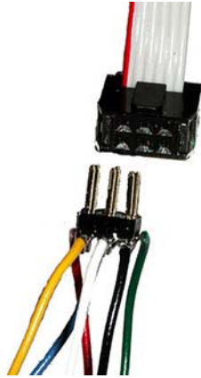
Figure 4: Dual 6-pin Header wires added.
